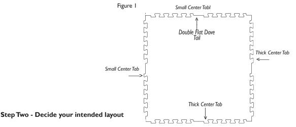
Tuff-n-Easy tiles may be laid in straight rows and columns or in a brick pattern offsetting either the rows or the columns by 50%. Since the seams do not ordinarily show, it is unlikely that after the tiles are installed that you will be able to detect which pattern was chosen. There is some locking benefit to the offset brick pattern.
